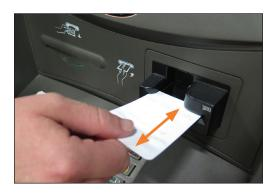
Insert card reader cleaner directly into card reader as you would a credit or debit card. Insert and remove several times.
